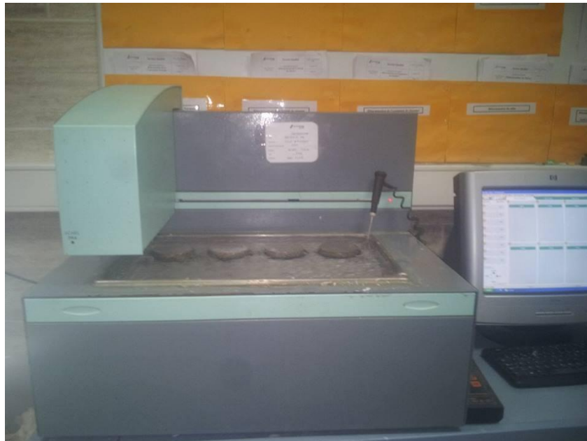
Figure III-10: Appareil Vicat
