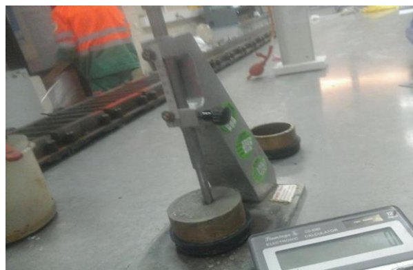
Figure III-9: appareil vicat
